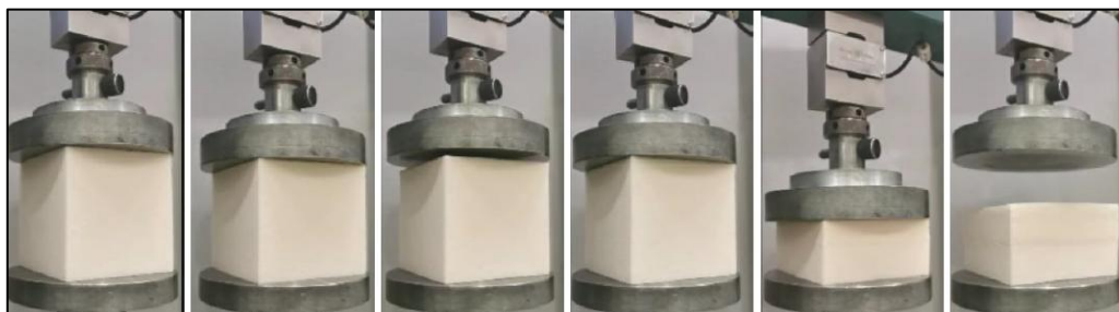
Figure 5: Pictorial image of foam compression test
