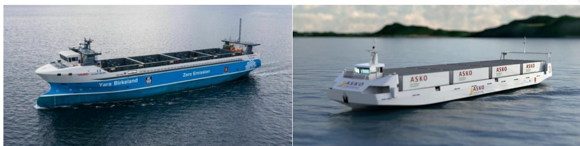
Figure 1. Yara Birkeland (left) and one of the ASKO barges (right). The Yara Birkeland is a battery-powered small container vessel owned by Yara International. Operating between Herøya and Brevik in Norway, it carries fertilizers and chemicals. The ASKO barges are battery-powered barges designed to transport containers across the Oslo fjord, between Horten and Moss in Norway. Both Yara Birkeland and the ASKO barges aim to reduce carbon emissions and road traffic by replacing diesel-powered truck transport.
