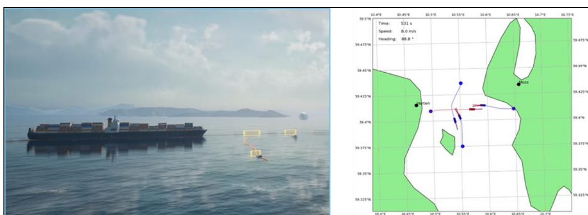
Figure 7. Example screenshots of simulator-based testing of ANS systems. High fidelity (3D game engine based) simulator (AI Livesim, 2018) for testing of external situational awareness system (left), and a simplified (2D) low fidelity simulator (Karolius et al., 2024b) for high volume testing of collision and grounding avoidance systems (right).
