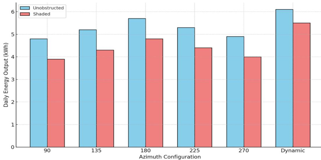
**Figure 10** Comparative visualization of daily energy output across various azimuthal configurations under both unobstructed and shaded conditions
