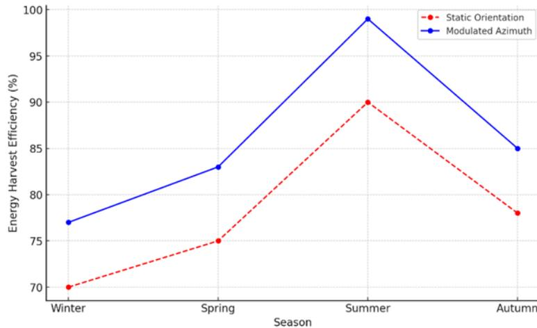
**Figure 5** Seasonal trends in PV efficiency through azimuth modulation
