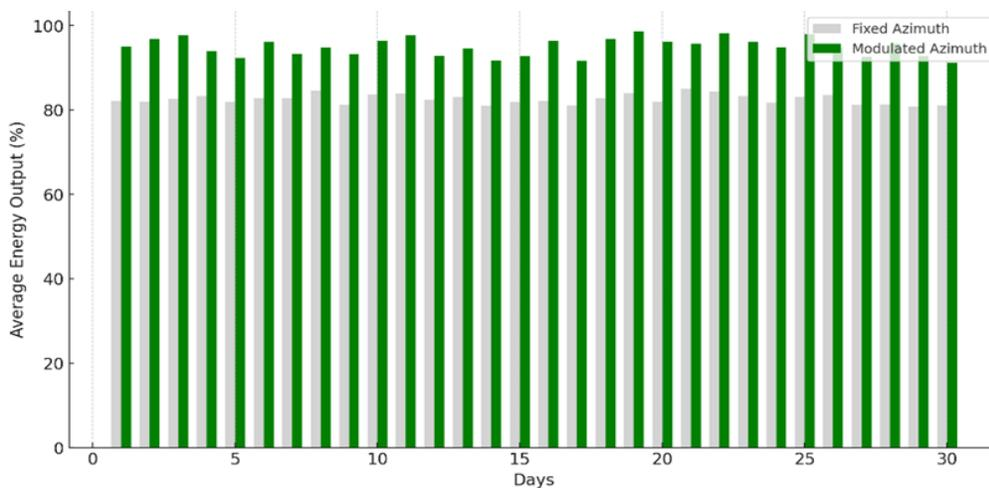
Figure 4 Comparative efficiency of fixed and dynamically modulated azimuth configurations based on simulated daily energy yield using ENERGY3D
