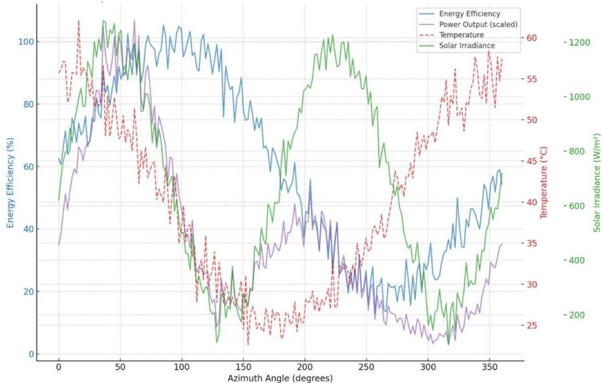
**Figure 6** Impact of azimuth angles on PV performance metrics
