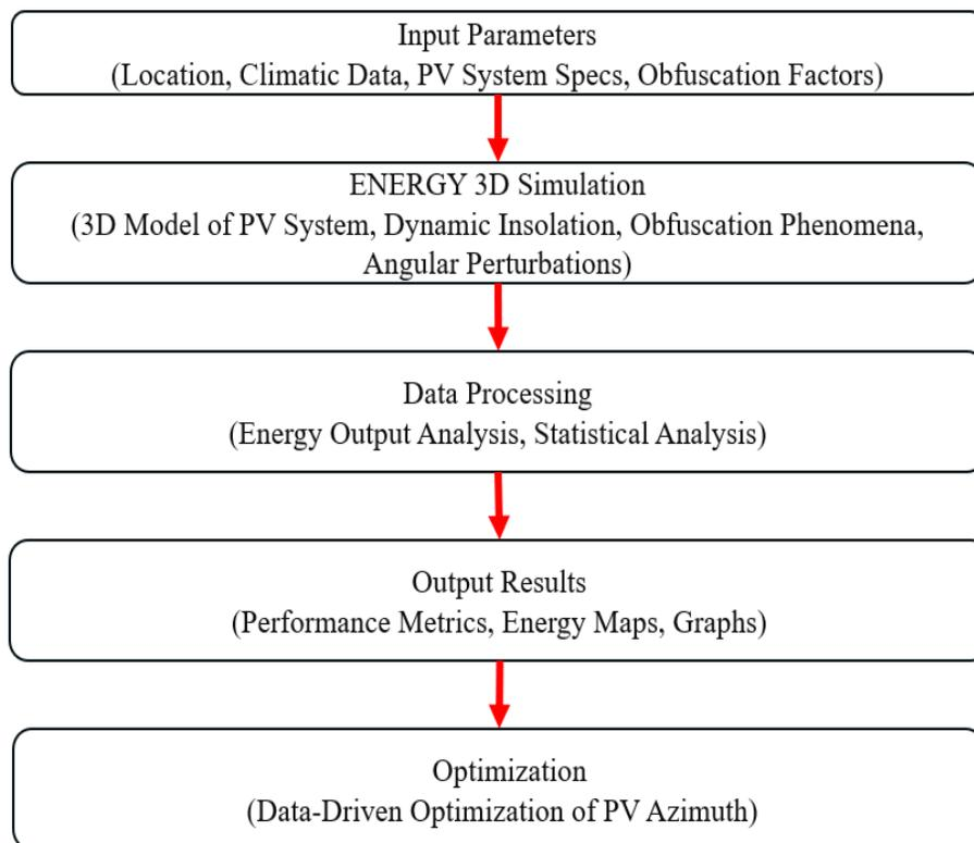
**Figure 2** Methodological framework for analyzing azimuthal perturbation effects on PV energy yield using ENERGY3D
