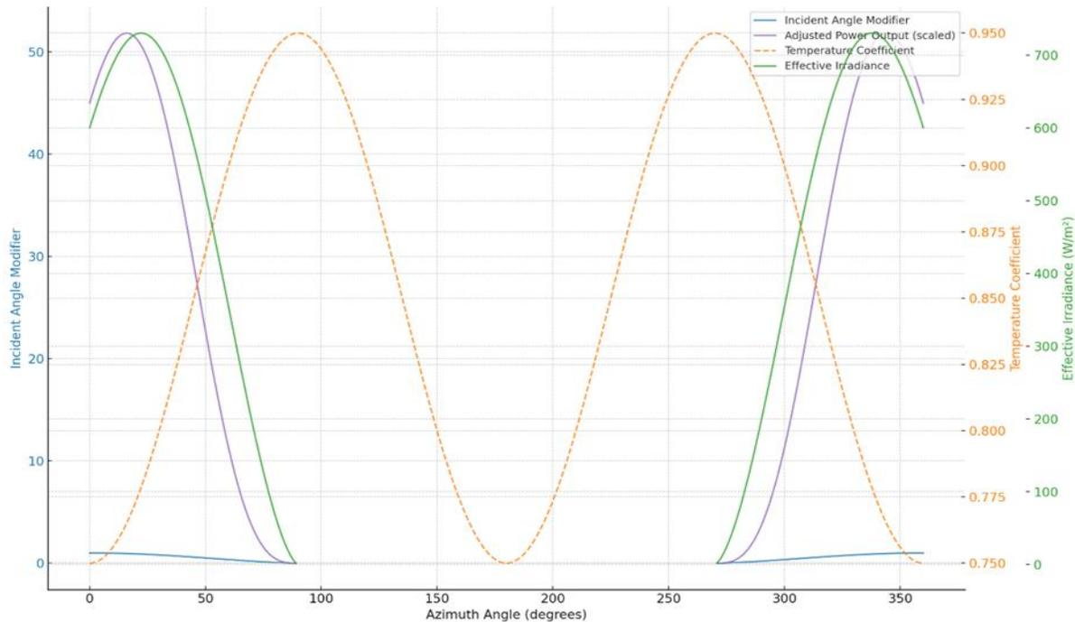
**Figure 7** The intricate relationships between PV angular modulation and various efficiency-influencing parameters
