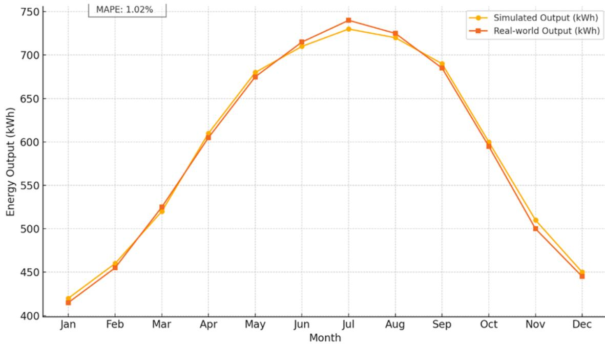
**Figure 9** Comparison between the Energy3D simulation results and the real-world output data
