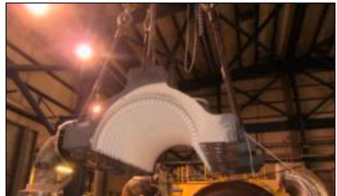
Fig. 8. High-pressure steam turbine casing.
