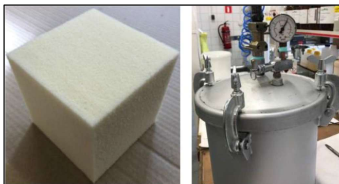
Figure 3: Foam test specimen shown left, pressure vessel shown right.
